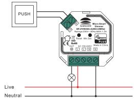
**NOTE:** Switch connected to the S1 terminal activates the basic functionality of the dimmer (turning the light on/off, dimming) and starts the inclusion/exclusion mode (Add/Remove).
