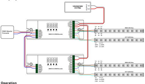
By holding button Back + Enter together at the same time over 5 seconds until the display go off, it will restore default settings.
