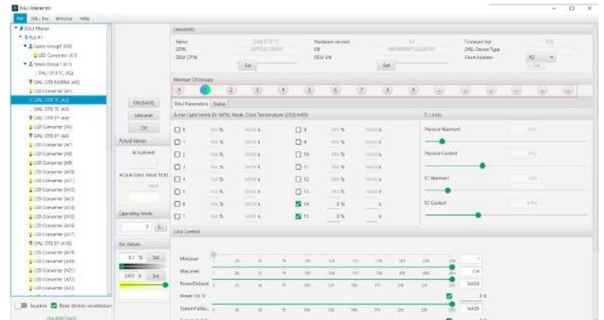
Figure 7 DALI Group Configuration for DT8 Tc Device
