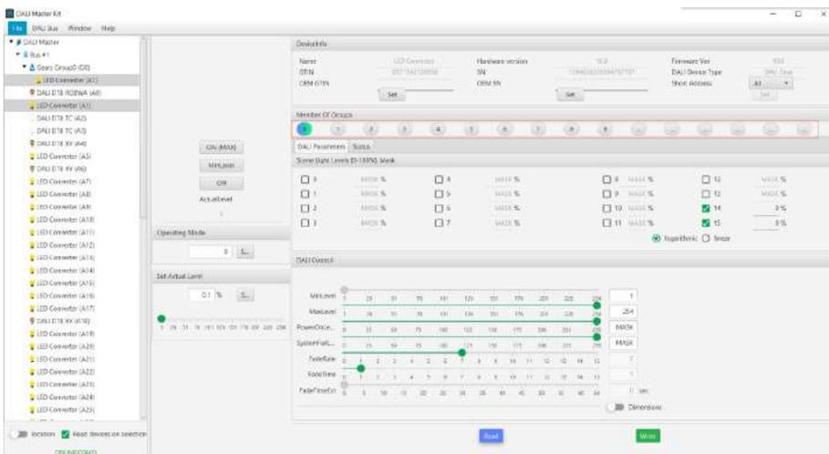
Figure 6 DALI Group Configuration for DT6 Device
