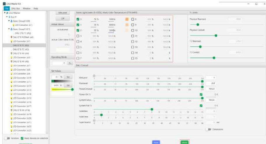
Figure 11 DALI Scene Configuration for DT8 Tc Device
