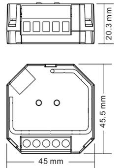
This phase dimmer adopts trailing edge dimming (reverse phase control), please make sure the connected loads support reverse phase control. Please refer to the user manual of the load or consult the supplier of the load.
