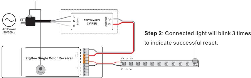
**Step 2:** Connected light will blink 3 times to indicate successful reset.
