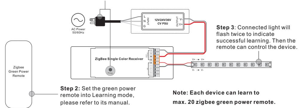
**Step 3:** Connected light will flash twice to indicate successful learning. Then the remote can control the device.
