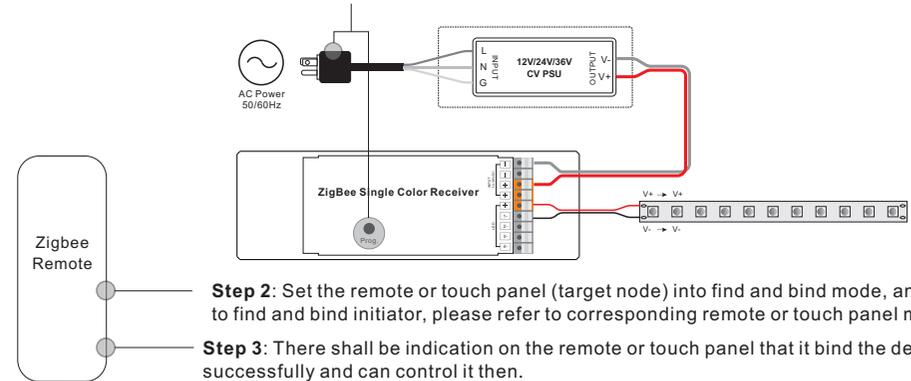
**Step 2:** Set the remote or touch panel (target node) into find and bind mode, and enable it to find and bind initiator, please refer to corresponding remote or touch panel manual.
